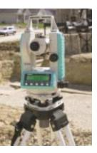
measurement capabilities of the Nikon NE-100 and NE-101 theodolites. Large, easy-to-identify buttons provide one-button operation for key functions. A large text display area makes information easy to read and use on the job. This design provides for a very short learning curve and utilization within a matter of minutes.
